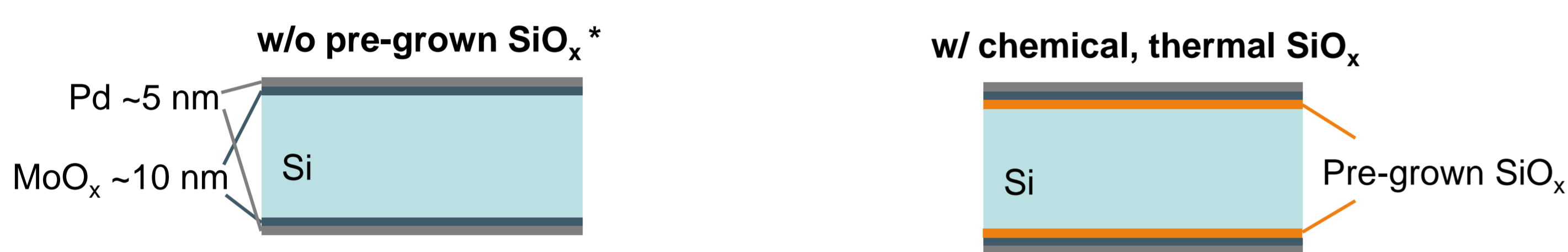
Figure 2. Schematic diagrams showing symmetrical lifetime structure used for J_0 extraction. (* a thin SiO x layer is still formed when depositing MoO x on HF dipped c-Si)
